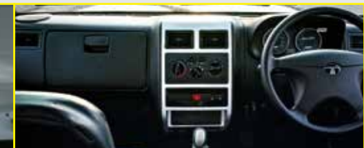
HVAC (Heating, Ventilation and AC)
